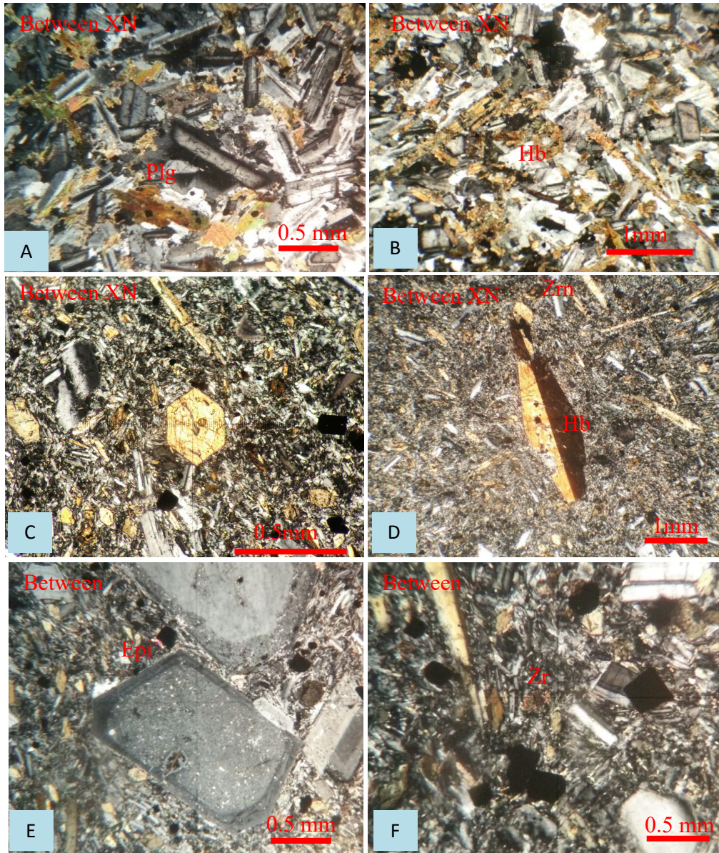
Figure 9: (A) Biotite and plagioclase in microdiorite (B) Anhedronal hornblende in microdiorite (C, D) Euhedral and twinned basal section hornblende in lamprophyre (E) Euhedral zoned plagioclase in lamprophyre (F) Euhedral four-sided pyrite mineral in lamprophyre
